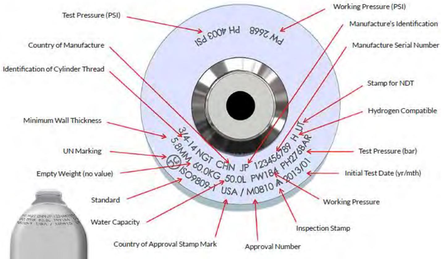
**TOP ROW** - Manufacturing marks such as the cylinder thread type, the country of manufacture, and the serial number assigned by the manufacturer.
